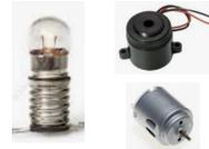
**Components** we will use are: cells or batteries, wires, bulbs, buzzers and motors. A switch can be added to a circuit to turn the **component** on and off by opening or closing the circuit.
